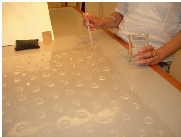
Fig. 13. Disposable pipettes dispensing the isinglass liquid into disk shapes to be dehydrated and stored for future use
