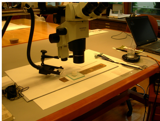
Fig. 11. Consolidating the paint layer with the aid of the binocular microscope
