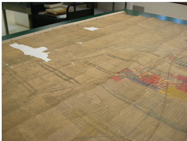
Figs. 12–13. Front of map before mending (left). Front of map after mending showing white muslin patches (right)
