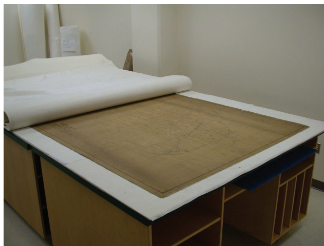
Fig. 11. Map between polyester webbing and felt after humidification and flattening
