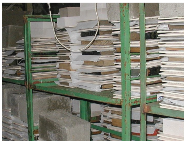
Fig. 7. Books stacked between unglazed ceramic tiles in kiln, Czech Republic
