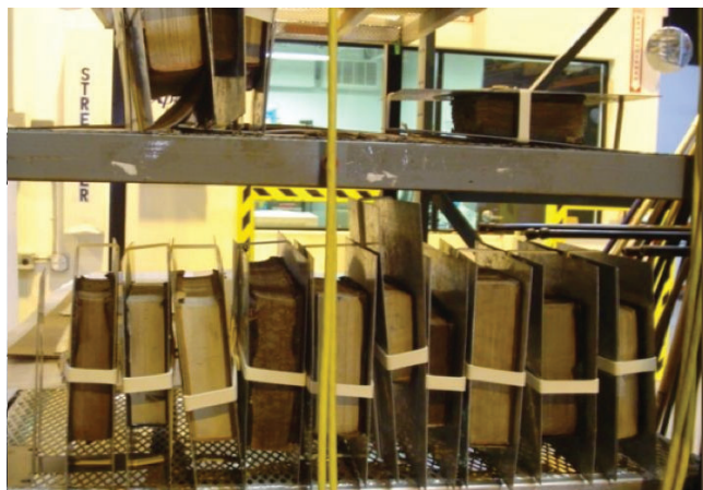
Fig. 5. Books on wire racks prepared for vacuum freeze drying, Belfor USA
