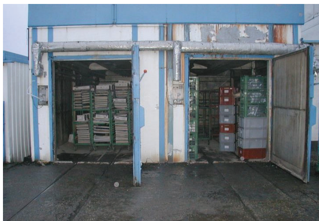
Fig. 6. Wood-drying kiln adapted for thermal drying, Czech Republic
